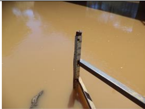
Plate 4.5: The first staff gauge at Perkera 2EE07, a check reading taken during the field visit to site was 0.56 m corresponding.
