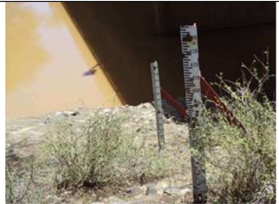
Plate 4.6: The second and third staff gauges at Perkera 2EE07
